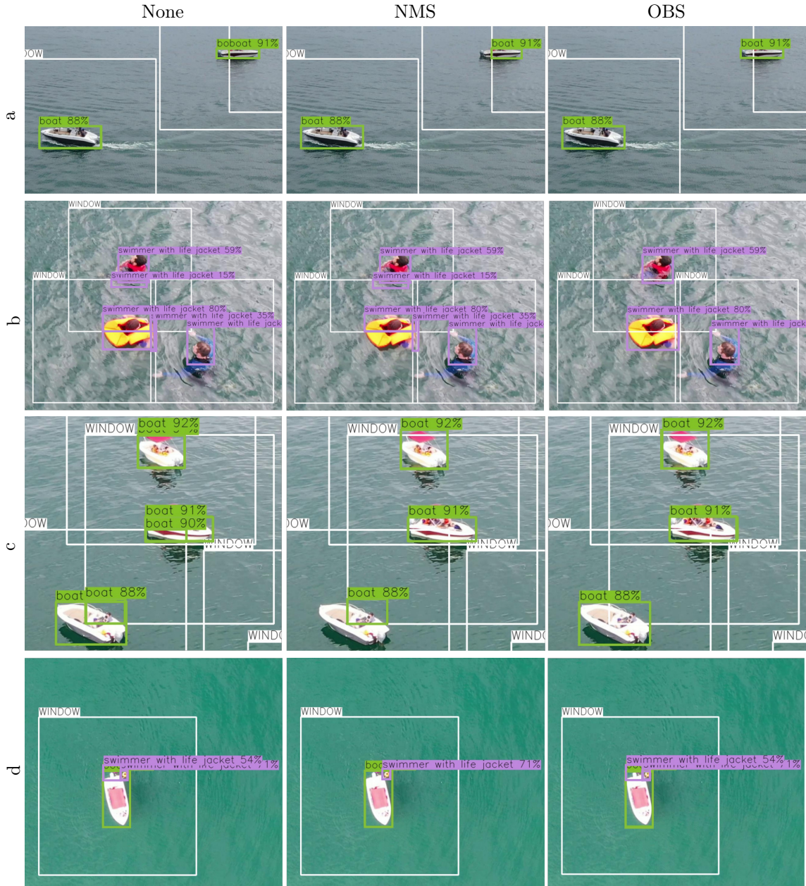
FIGURE 6.7: Qualitative comparison of no global filtering (None), NMS, and OBS . Without global filtering, many false positives remain. NMS retains a high-confidence partial detection, incorrectly suppresses a full detection, and fails to remove all fragmentary boxes. In contrast, OBS effectively eliminates all false positives without causing false negatives, preserving all correct detections. Additionally, because of the low IoU threshold, NMS suppresses a correct detection that OBS correctly retains by leveraging the detection window coordinates.
