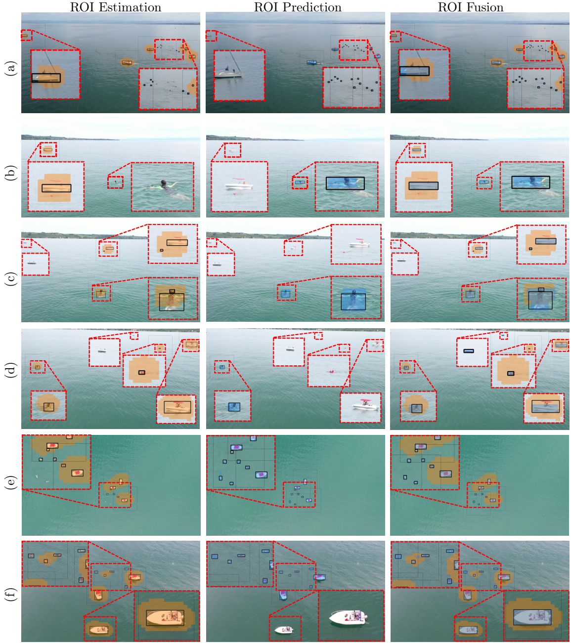
FIGURE 5.7: Example results comparing segmentation-based detection (first column), tracking-based detection (second column), and the proposed method that integrates ROIs from both segmentation and tracking modules (third column). Blue regions indicate predicted ROIs, orange regions represent estimated ROIs, thin black boxes show detection windows, and thick black boxes denote detected objects. All examples are drawn from the SeaDronesSee [132] dataset. In the proposed architecture, the ROI Estimation and Prediction Branches operate in coordination rather than independently; therefore, the ROIs shown in the third column are not a simple union of those in the first and second columns.
