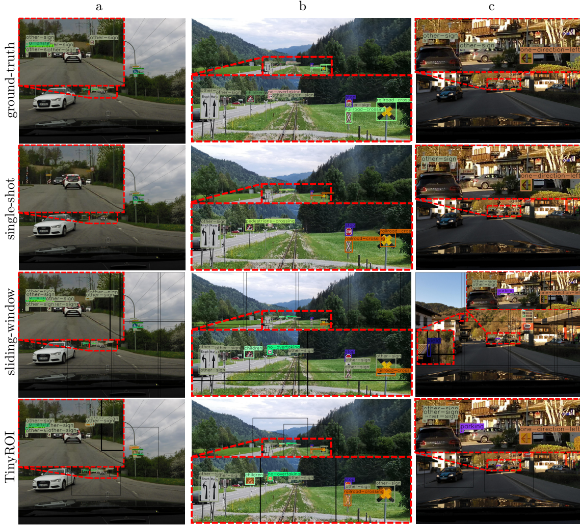
FIGURE 4.8: Qualitative results comparing ground-truth annotations with single-shot detection using downsampling, and window-based approaches: naive sliding-window and the proposed TinyROI system incorporating a learned ROI Estimation Module. Black rectangles indicate detection windows, while orange regions in the TinyROI row represent returned ROIs. Single-shot detection often misses tiny objects, which can be recovered by full-resolution inference in both the sliding-window and TinyROI approaches. However, the sliding-window method introduces more false positives, likely due to object fragmentation and complex backgrounds. In contrast, the learned ROI Estimation Module in TinyROI acts as an initial filtering step, helping to reduce false positives. While this may occasionally result in missed detections, the significantly reduced processing time justifies the trade-off.
