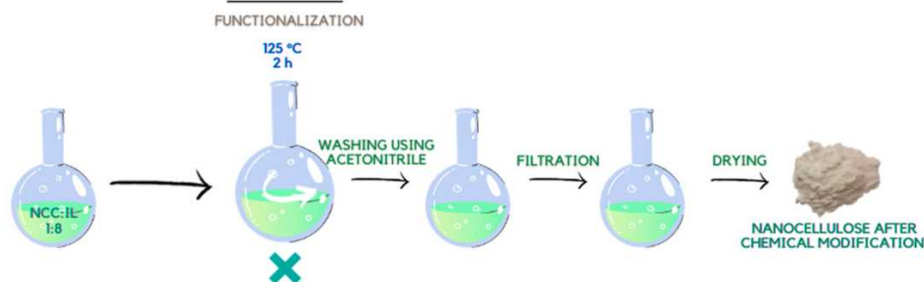
Figure 10. Scheme of chemical modification of nanocellulose using IL's.
