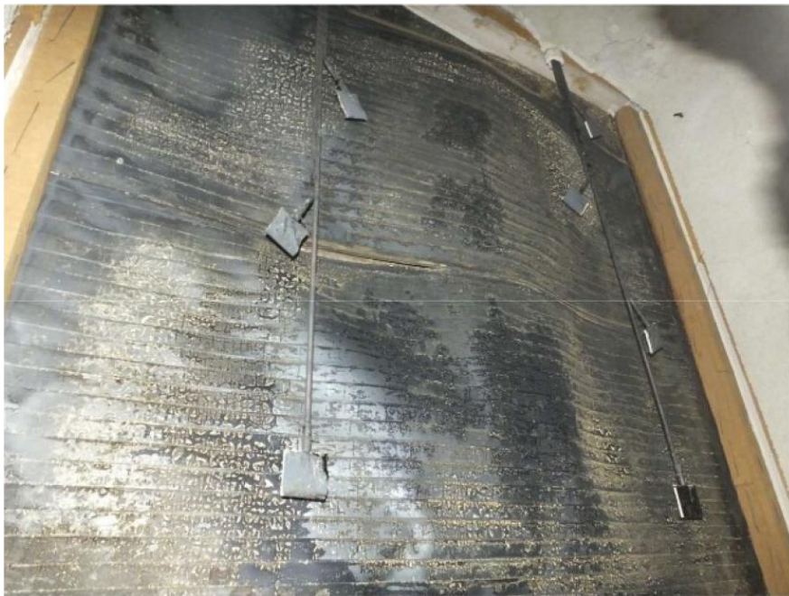
Figure 120. Condition of the tested wall specimen – heated side of test 4' at the end of the test.
