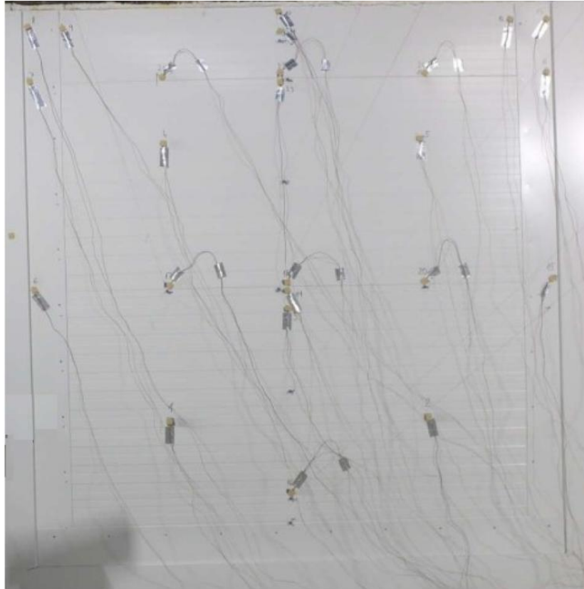
Figure 117. Initial setup of the tested wall specimen - unheated side of test 4'.
