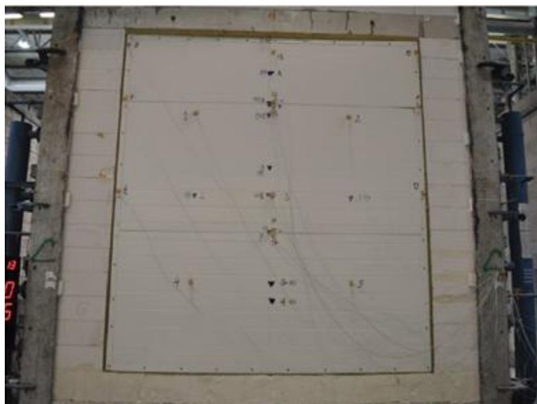
Figure 114. Condition of the tested wall specimen – unheated side of test 1' at 30 minutes.
