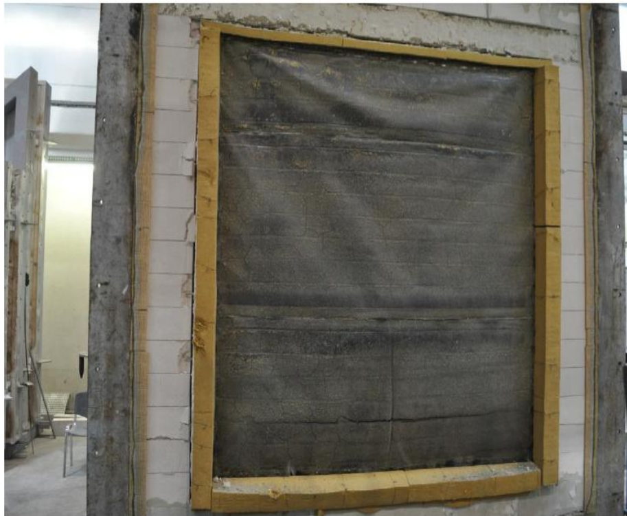
Figure 116. Condition of the tested wall specimen – heated side of test 1' at the end of the test.
