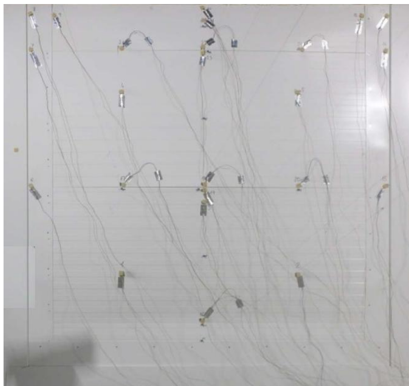
Figure 118. Condition of the tested wall specimen – unheated side of test 2' at 95 minutes.
