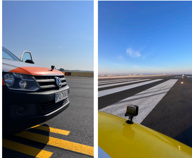
Figure 3-2 The concept of the FOD detection system (camera mounted on the front of a car moving along the runway at the Poznań–Ławica Airport) [37]
