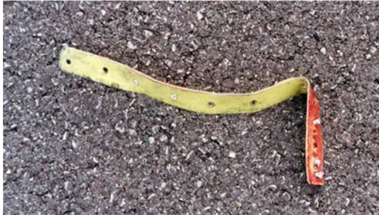
Figure 1-6 Example FOD, the metal strip suspected of piercing the Concorde tyre [16]
