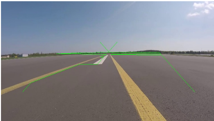
Figure 4-9 Result of running a program for line detection based on an edge detection algorithm [30]
