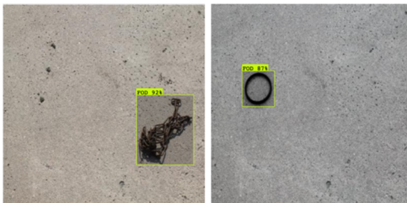
Figure 3-12 Results of FOD detection using YOLOv5 and PUT dataset [38]
