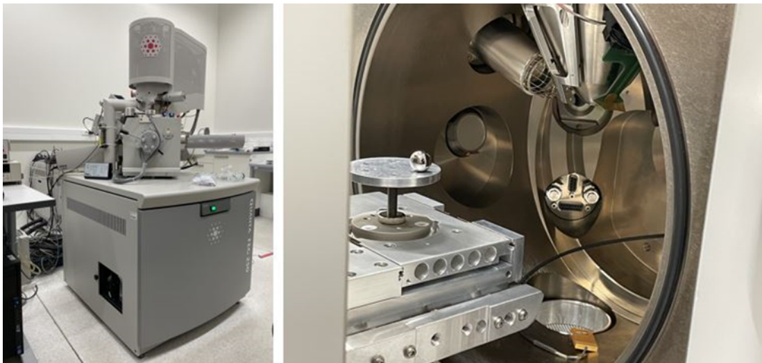
Fig. 3.7 Quanta FEG 250 used for most SEM microscopy and EDS spectroscopy tasks in this thesis, picture of the microscope column and close view to the microscope chamber with detectors
