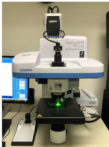
Fig. 3.11 Raman spectroscope, a with sample in the optical microscope, green laser incident light for Raman scattering and motorized sample table visible
