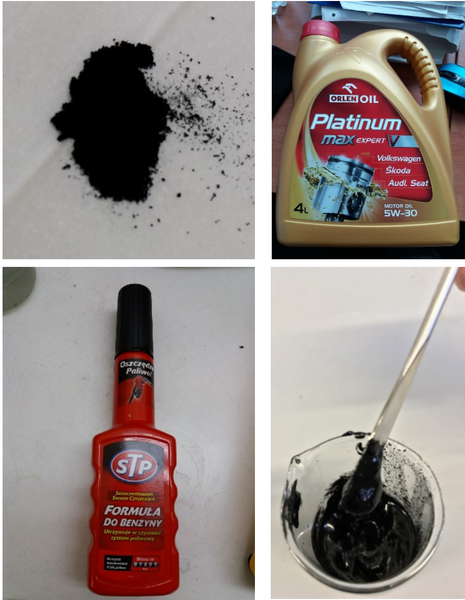
Fig. 3.1 Carbon nanotubes (CNTs), engine lubricating oil, surfactant and experimental grease as a product, examples from the own experiment
