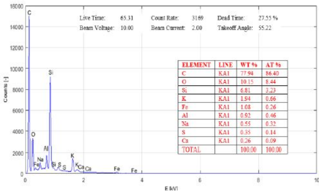
Fig. 5.7 EDS spectroscopy results for the surface of the CNT layer on the piston dismantled after the engine tests were completed
