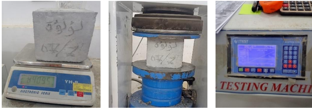
Figure 7.25 RMC compressive strength f_c (MPa) test results for the sample at the SCBP on 7 th July 2021, for the reinforced beams and slab of the first floor, at age 28 days [Researcher].
