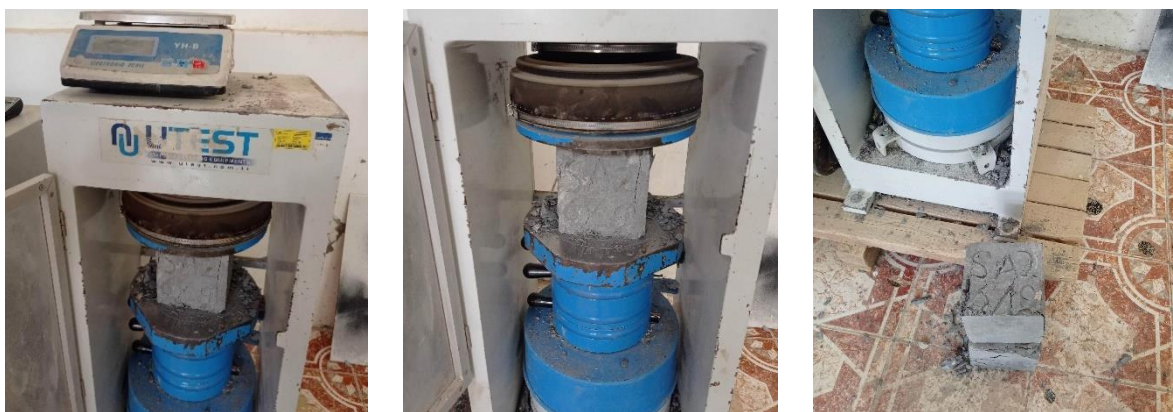
Figure 6.18 The compressive strength f_c (MPa) of RMC at the laboratory at 28 days age [Researcher].
