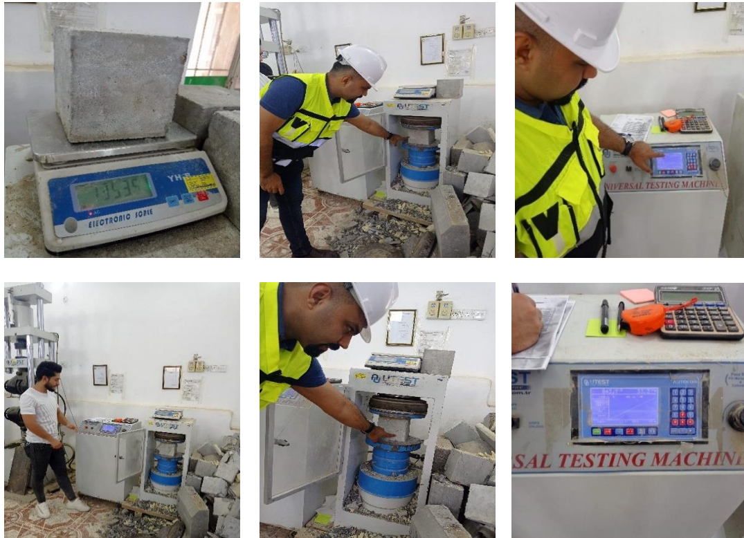
Figure 7.26 RMC compressive strength (MPa) test results for the sample at the SCBP on 27 th July 2021, for the reinforced beams and slab of the first floor, at age 28 days [Researcher].
