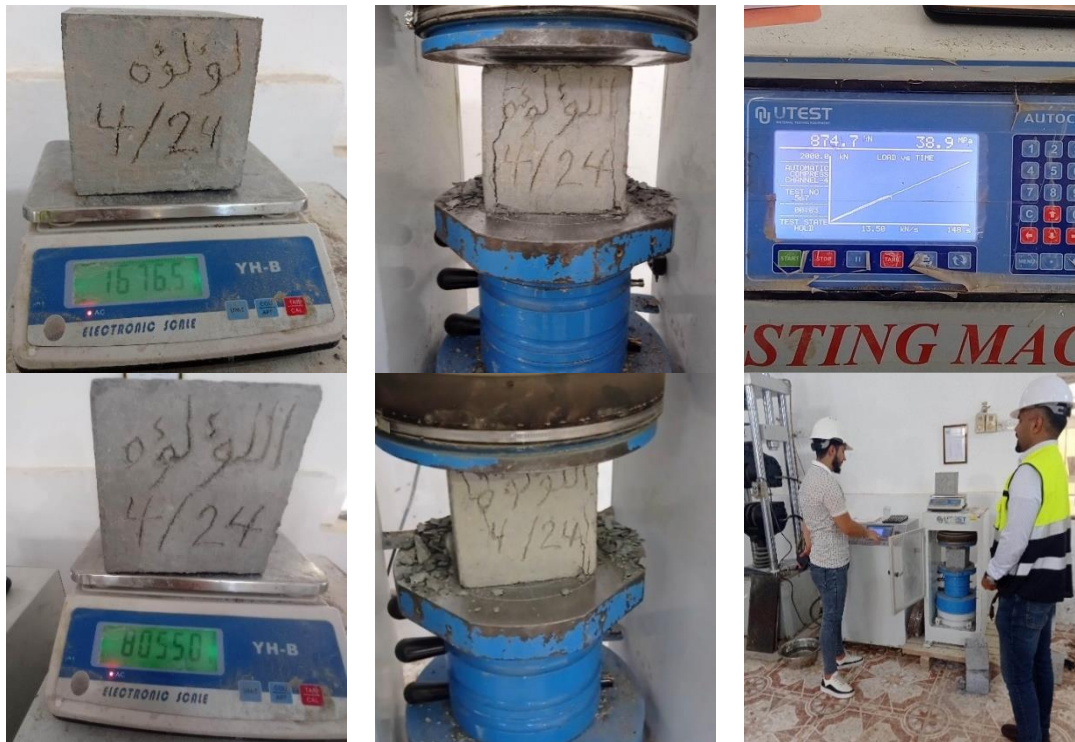
Figure 7.21 RMC compressive strength f_c (MPa) test results for the sample at the SCBP on 24 th April 2022, for the reinforced beams and slab of the second floor, at age 28 days [Researcher].
