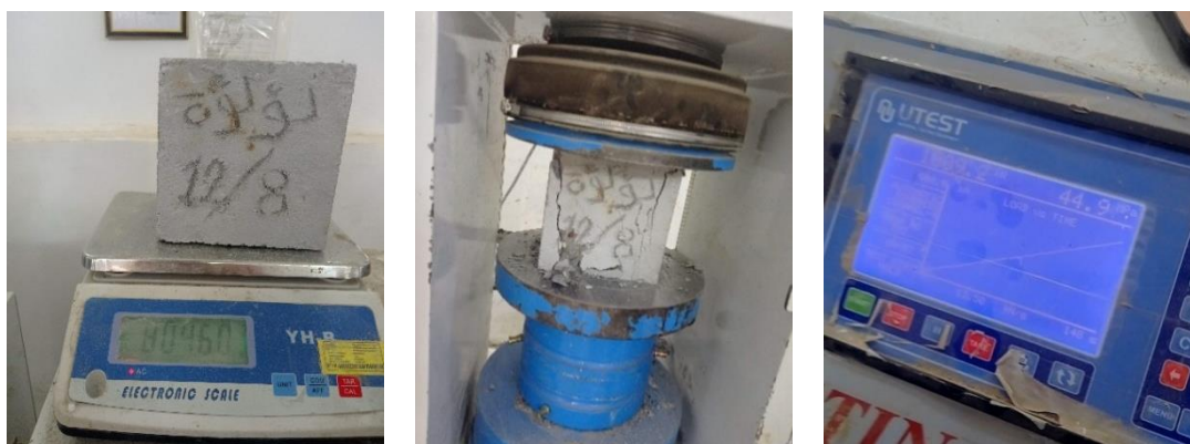
Figure 7.22 RMC compressive strength (MPa) test results for the sample at the construction site on 8 th December 2021 for the second-floor reinforced columns at age 28 days [Researcher].
