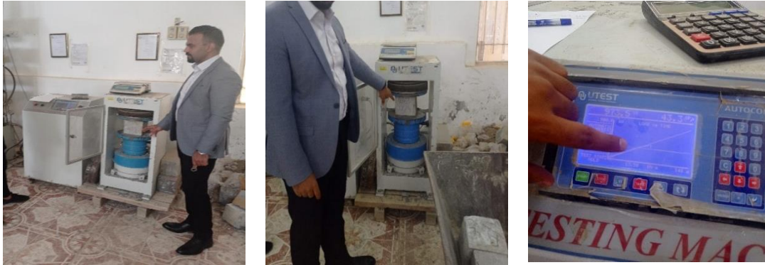
Figure 7.23 RMC compressive strength (MPa) test results for the sample at the SCBP on 9 th December 2021, for the second-floor reinforced columns, at age 28 days [Researcher].
