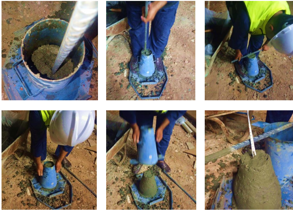
Figure 7.10 The slump test of the RMC mix at the construction site for the samples taken on 27 th July 2021 after reducing the temperature of the RMC mix [Researcher].
