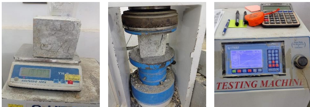
Figure 7.24 The RMC compressive strength (MPa) test results for the sample at the SCBP on 1 st July 2021 for the reinforced beams and slab of the first floor at age 28 days [Researcher].
