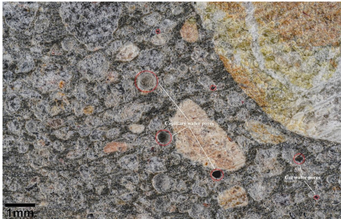
Figure 7.38 RMC sample photographed with 1mm accuracy, showing porosity of 20.49 % and air content of 3.6 %, in a mix with a water/cement ratio of 0.5, achieving a compressive strength 44.9Mpa [Researcher].
