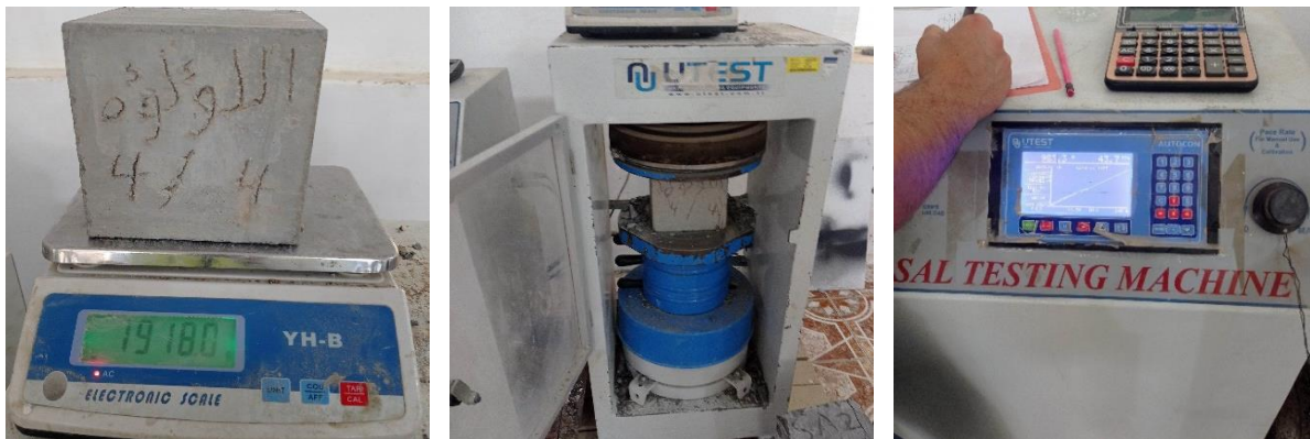
Figure 7.20 RMC compressive strength (MPa) test results for the sample at a construction site on 4 th April 2022 for the reinforced beams and slab of the second floor, at age 28 days [Researcher].
