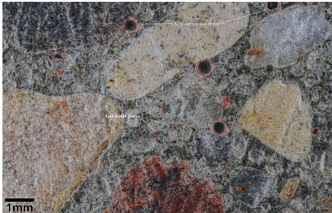
Figure 7.37 RMC sample photographed with 1mm accuracy, showing porosity of 19.22 % and air content of 2.8% in a mix with a water/cement ratio of 0.5, achieving a compressive strength of 43.7 Mpa [Researcher].
