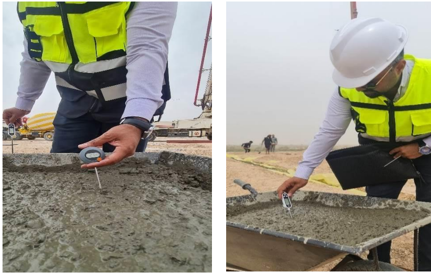
Figure 7.2 RMC temperature samples were measured by two thermometers with water-cement of ratio 0.5 Portland cement (type I) and different weather temperatures [Researcher].
