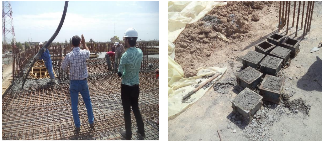
Figure 6.17 RMC compressive strength test samples for the ground floor slab (3 second-stage cubes) at 28 days [Researcher].
