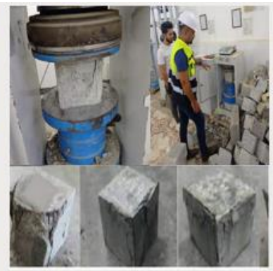
Figure 1.7 Decreasing strength Compressive Strength test failure [Researcher].
