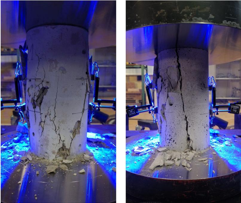
*Fig. 9.27 One of the specimens after several loading-unloading cycles.*
