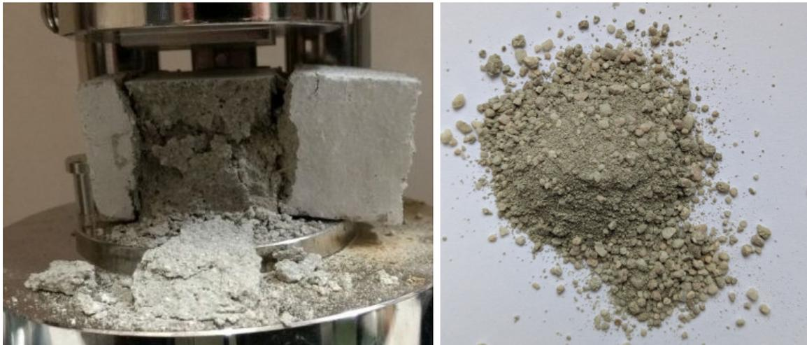
*Fig. 4.14 Degradation of standard mortar after heating to 1000 °C (a) one day after heating, (b) one month after heating (own research).*
