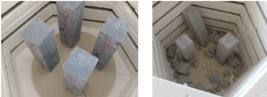
Fig. 9.6 The results of preliminary tests. Specimens without PP fibres and oven drying: (a) before and (b) after heating to 600 °C at a rate of 5 °C/min (Szymkuć et al. 2018a).
