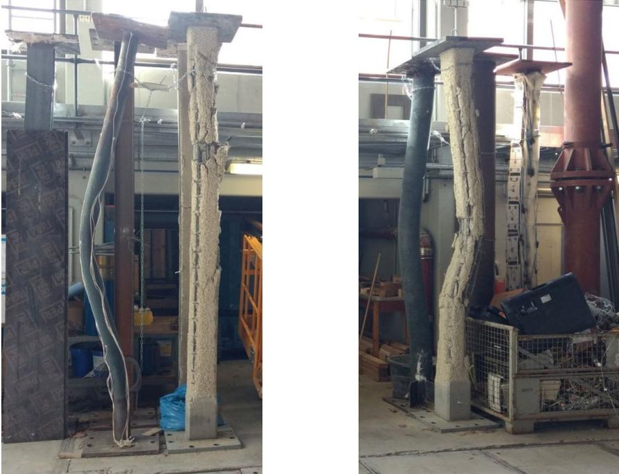
Fig. 1.4 CFST and RC columns after fire resistance tests. Extensive damage to concrete cover in RC columns is visible. BAM, Berlin (photo: Wojciech Szymkuć).
