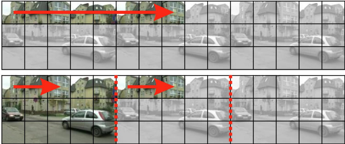
Figure 6.2. HEVC coding order without (above) and with (below) tile encoding.
