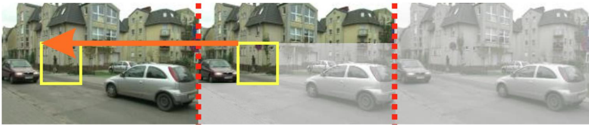
Figure 6.3. Long inter-view prediction vector derived by Intra Block Copy.
