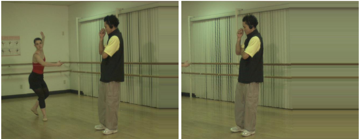
Figure 4.8. A real example of the problem with the misaligned fields of view after circular rectification, Breakdancers test sequence. View number 4 (left) is slightly misaligned, and view number 6 (right) is significantly rotated towards the center of a circle but outside the center of the acquired scene.
