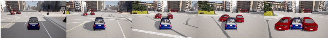
FIGURE 5.11: Sequence of frames from the scenario of diagonal parking in a 175cm wide parking place using episodic planner. Precise planning and superior path-tracking performance allow for parking in a place that has only about 8cm of theoretical slack.
