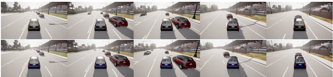
FIGURE 5.8: Sequences of frames from the scenario of parallel parking executed with the use of the sequential (top rows) and episodic planners (bottom rows).
