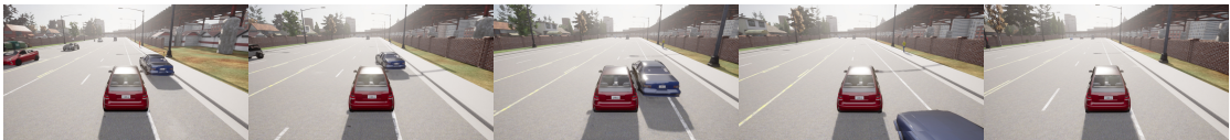
FIGURE 5.13: Sequence of frames from the high-speed collision avoidance using the episodic planner.
