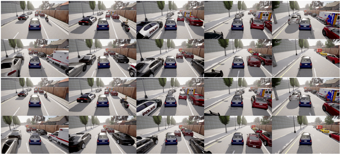
FIGURE 5.7: Sequences of frames from the scenario of passing densely parked vehicles executed with the use of the sequential (top rows) and episodic planners (bottom rows).
