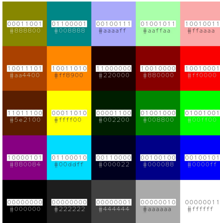
Figure 2.10: Example colours with their 8 bits colour descriptors (white rectangles), and RGB hex codes.
