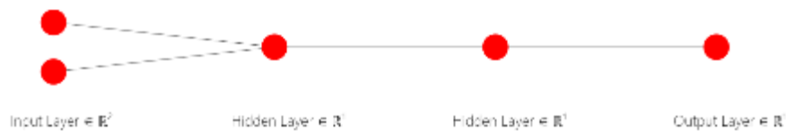
a. Base architecture with 2 hidden layer and one neuron in each layer
