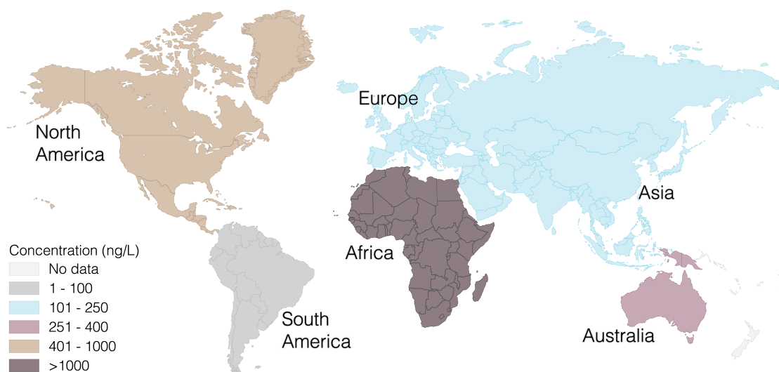
Fig. 3 Median concentration of antibiotics reported in municipal wastewater treatment plant influents on different continents. Adapted from Adeleye et al. (2022).
