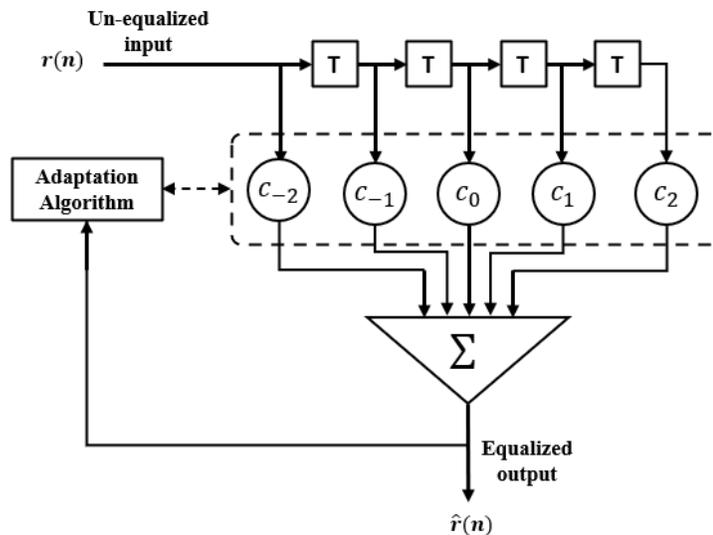
**Figure 5. 4 Basic structure of linear adaptive equalizer**
