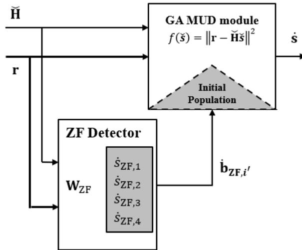
Figure 4. 2 SIC-inspired GA-MUD block diagram
