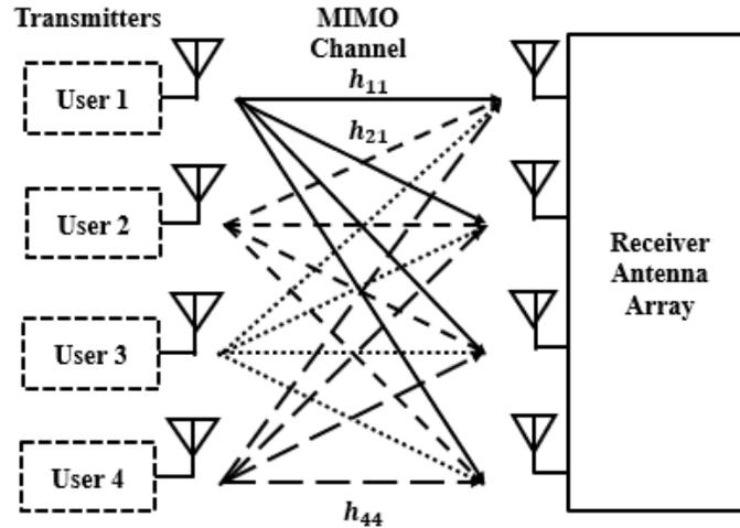
**Figure 3. 2 Schematic of general MU-MIMO communication system**
