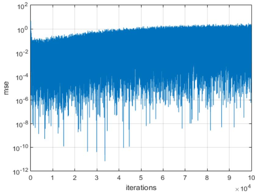
**Figure 5. 23 MSE vs iteration of the LMS at SNR = 35 dB and  $f_d = 3$  Hz in the case of 6-tap urban propagation model**
