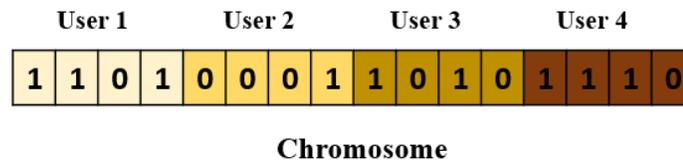
**Figure 3. 5 Chromosome representing a candidate multi-symbol for which  $\check{b}_1 = (1101)$ ,  $\check{b}_2 = (0001)$ ,  $\check{b}_3 = (1010)$ ,  $\check{b}_4 = (1110)$  [KK18, Kha17]**
