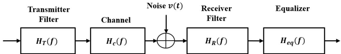
**Figure 5. 3 An equalization system block diagram**
