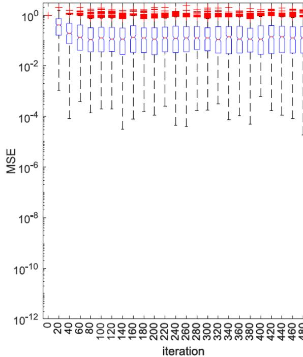
**Figure 5. 21** Box plots of convergence characteristics of the RLS at SNR = 35 dB,  $f_d = 0$  Hz in the case of typical urban area 6-tap channel
