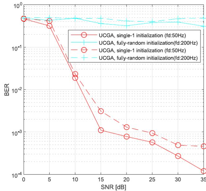
**Figure 5. 16 Comparison of different population initialization methods: fully-random initialization and single-1 initialization; assumed typical urban area 6-tap channel model with specific Doppler shifts:  $f_d = 50$  Hz (red curves) and  $f_d = 200$  Hz (blue curves)**
