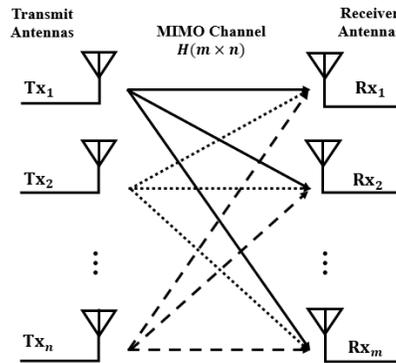
**Figure 3. 1 General schematic representation of a MIMO system utilizing  $n$  transmit antennas and  $m$  receiver antennas [JH07]**
