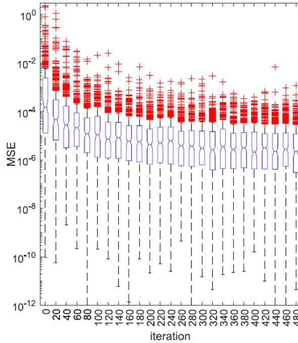
**Figure 5. 20** Box plots of convergence characteristics of UCGA at SNR = 35 dB,  $f_d = 0$  Hz in the case of typical urban area 6-tap channel
