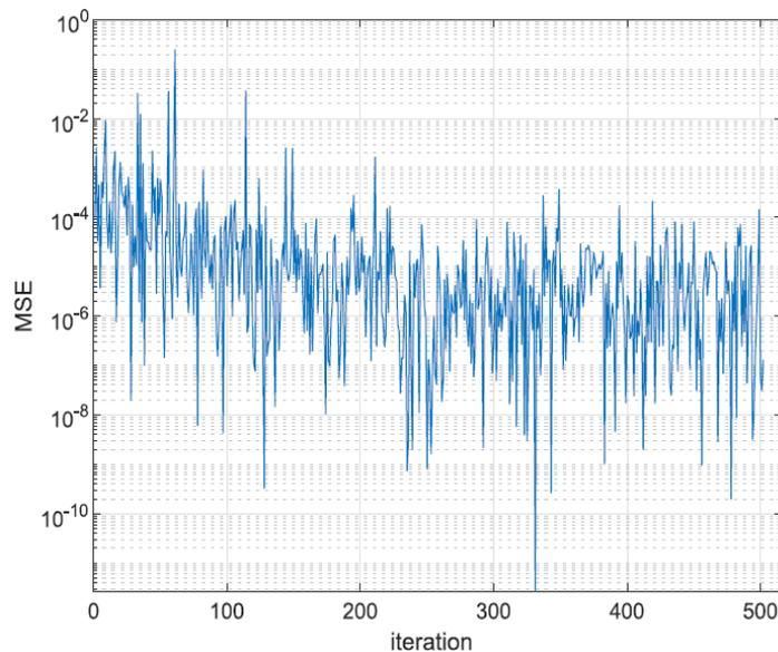
**Figure 5. 17** Convergence characteristics of UCGA at  $\text{SNR} = 35 \text{ dB}$ ,  $f_d = 0 \text{ Hz}$  in the case of typical urban area 6-tap channel
