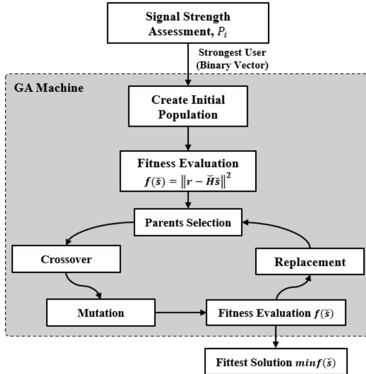
Figure 4. 4 GA machine cycle
