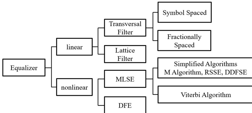
Figure 5. 2 Classification of the equalization structures
