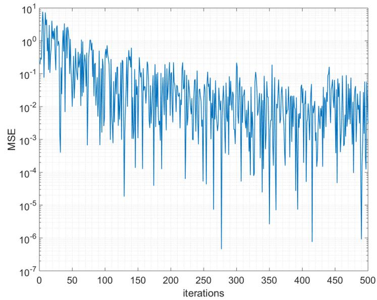
**Figure 5. 18** Convergence characteristics of the LMS at SNR = 35 dB,  $f_d = 0$  Hz in the case of typical urban area 6-tap channel
