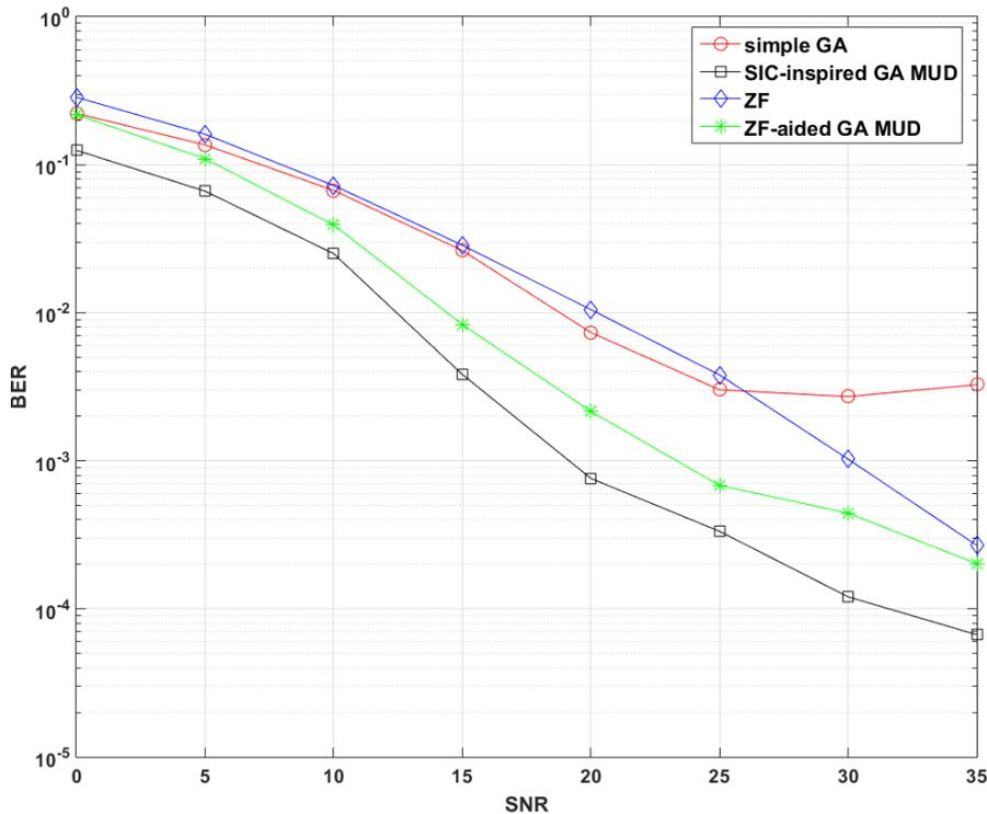
Figure 4. 5 BER vs SNR for the compared multi-user detectors
