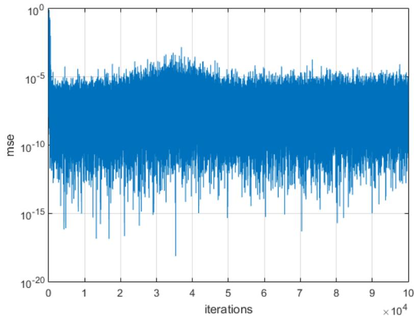
**Figure 5. 22 MSE vs iteration of UCGA at SNR = 35 dB and  $f_d = 3$  Hz in the case of 6-tap urban propagation model**
