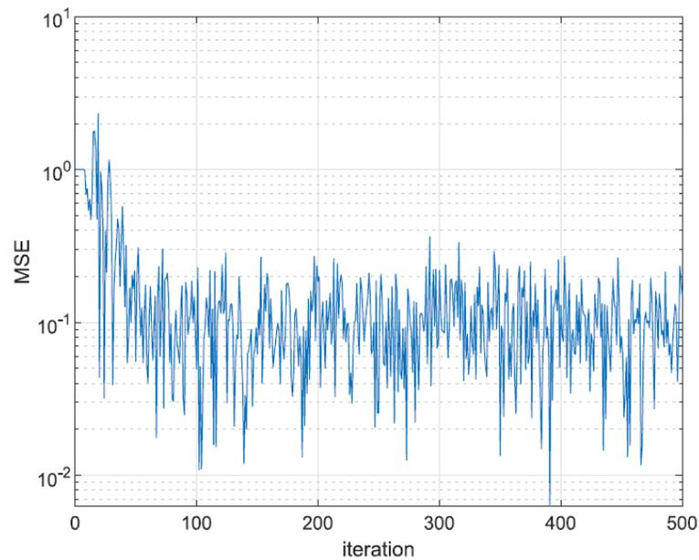
**Figure 5. 19** Convergence characteristics of the RLS at SNR = 35 dB,  $f_d = 0$  Hz in the case of typical urban area 6-tap channel
