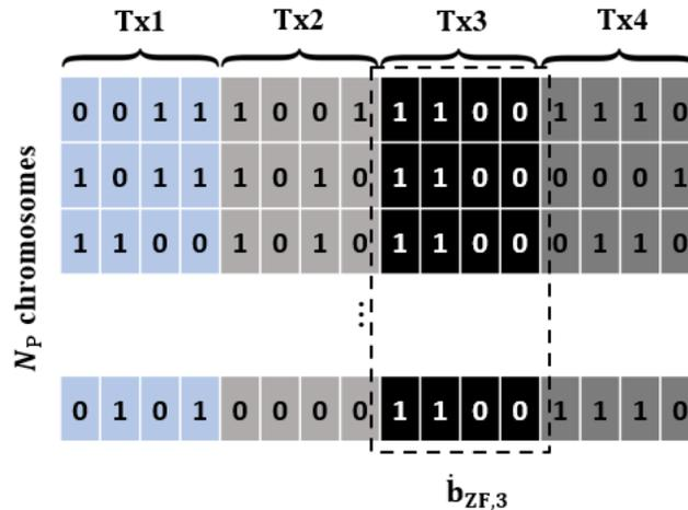
Figure 4. 3 Initial population in the case of 16-QAM modulation,  $i' = 3$ , and
