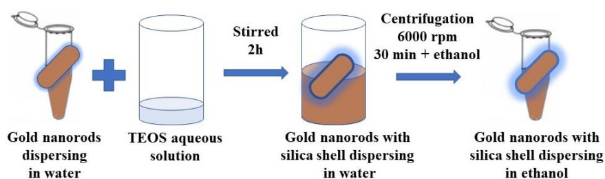
Scheme S2. Functionalization of Au-NRs with \text{SiO}_2 .
