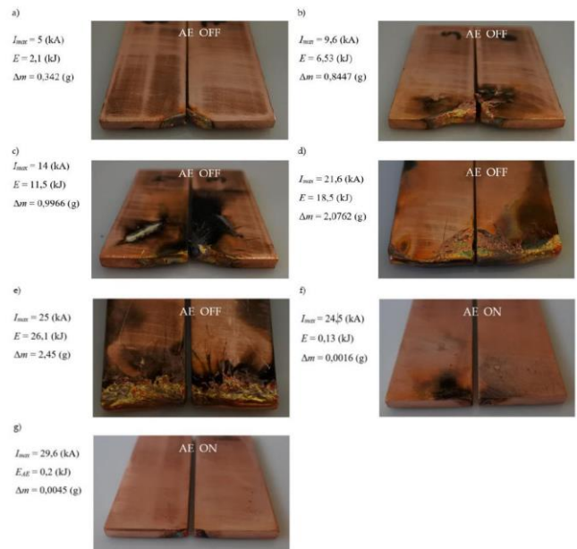
FIGURE 10. Erosion of the material of copper electrodes as a result of the action of an electric arc in a system without AE (AE OFF) and with (AE ON) an arc eliminator ( I_{max} – measured value of the interference current, E – calculated electric arc energy, \Delta m – measured material loss of both electrodes).
