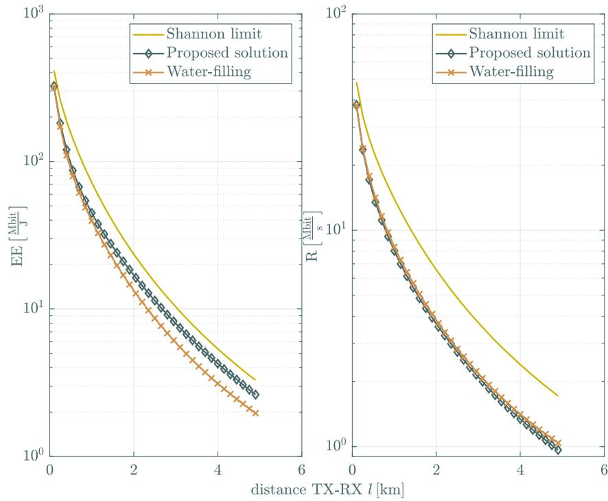
Figure 2.5: Energy efficiency (left) and throughput (right) versus the link distance.
