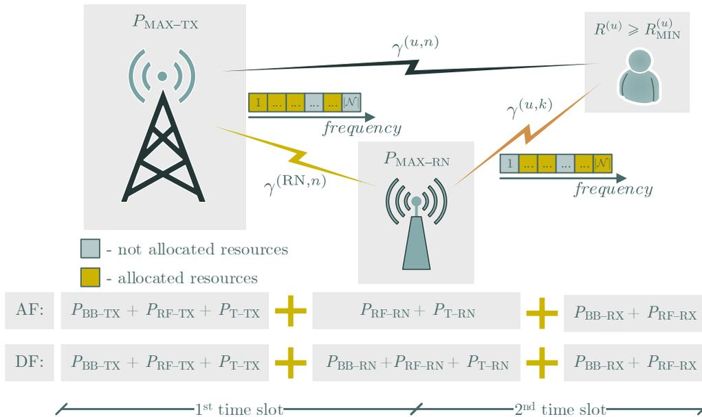
Figure 4.6: Transmission supported by the relay node, and the power consumption related to the amplify and forward and decode and forward relaying protocols, where  $\gamma^{(x,y)}$  determines the SNR value at the receiver  $x$  observed on subcarrier  $y$ .
