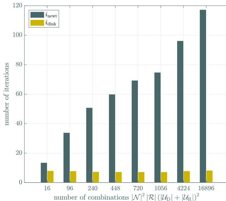
Figure 4.9: The mean number of iterations of the Newton and Dinkelbach method vs. number of combinations.
