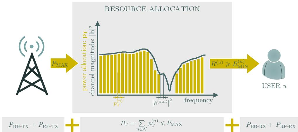
Figure 2.1: The single link scenario, where  $p_T^{(n)}$  determines the power allocated on SC  $n \in \mathcal{N}$ , the channel coefficient in the link is defined by  $h^{(u,n)}$  while  $R^{(u)}$  is the data rate achieved by user  $u$ . The variables related to the system constraints are denoted as  $P_{MAX}$  and  $R_{MIN}^{(u)}$  which define the maximum transmit power and the minimum data rate achieved by user, respectively.
