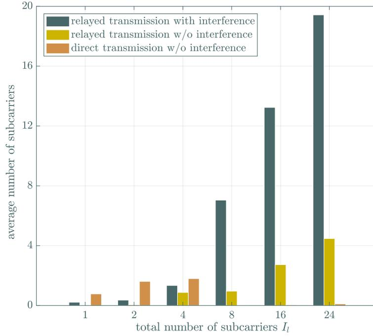
Figure 4.14: The mean of subcarriers used in a given transmission mode versus the total number of subcarriers.
