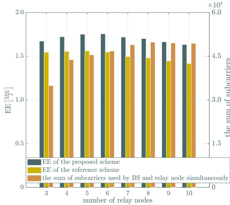
Figure 4.12: The energy efficiency of the proposed and reference schemes and the sum of SCs which have been used simultaneously by BS and the relay node in the second TS.
