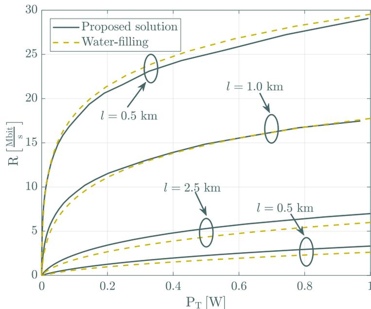
Figure 2.9: Throughput versus the total transmit power.
