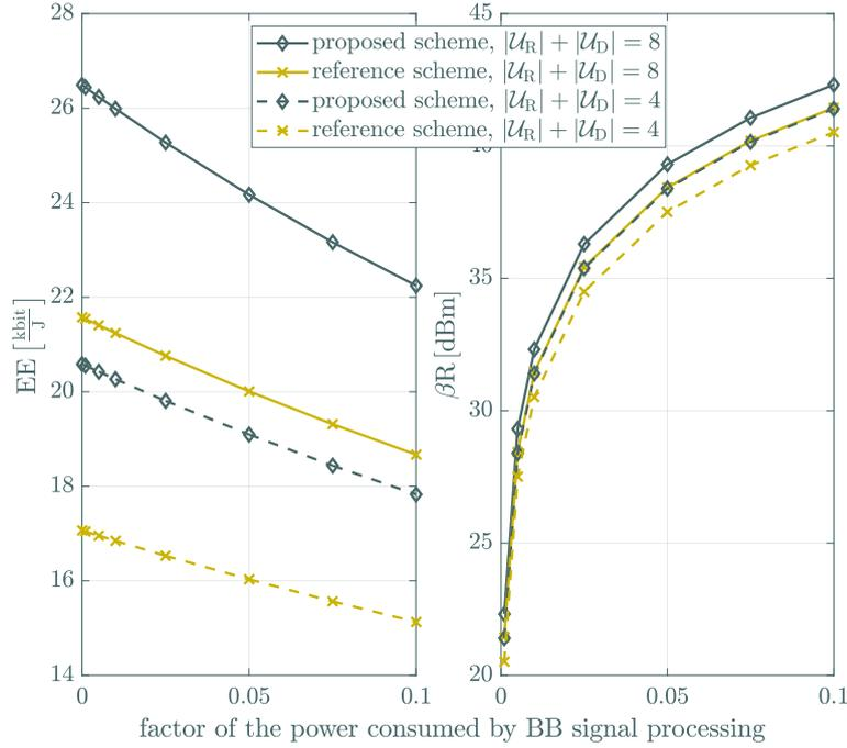
Figure 4.17: The energy efficiency and the power consumption of BB processing as a function of the factors  $\beta_R^{(u_R, r)}$  and  $\beta_D^{(u_D)}$  assuming that  $\beta = \beta_R^{(u_R, r)} = \beta_D^{(u_D)}$  for all  $k, m, n$ .
