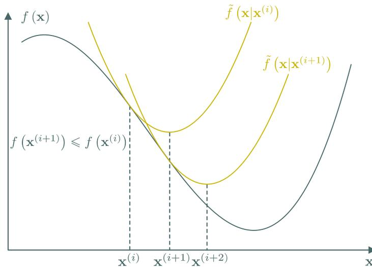
Figure 4.7: The illustration of the Successive Concave/Convex Approximation method.
