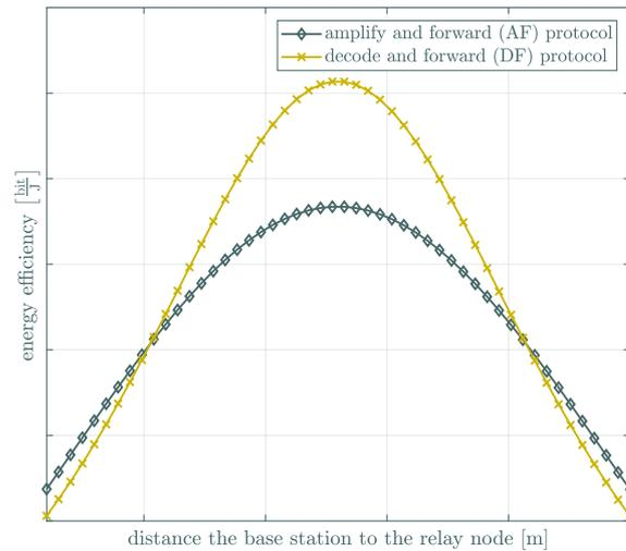
Figure 4.4: The energy efficiency against the distance from the base station to the relay node.
