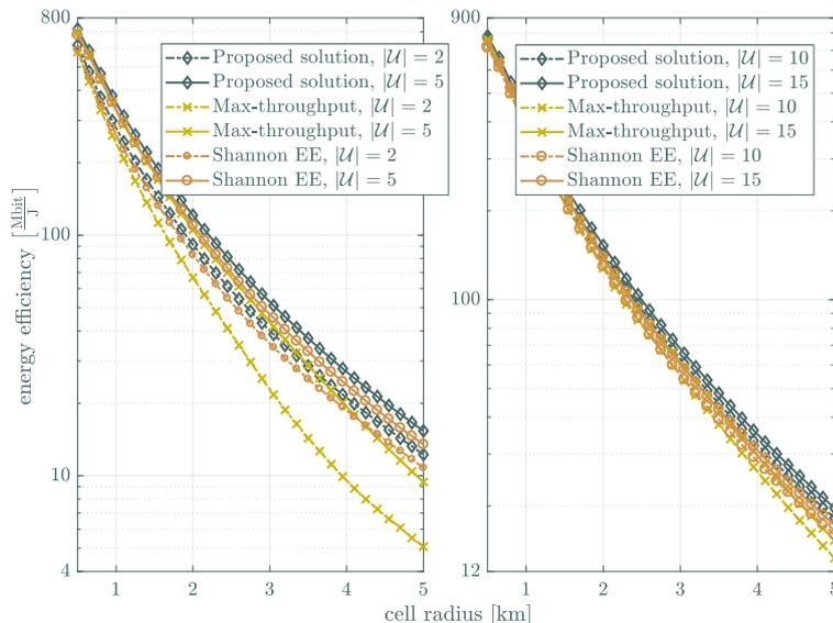
Figure 3.9: energy efficiency versus the cell radius.
