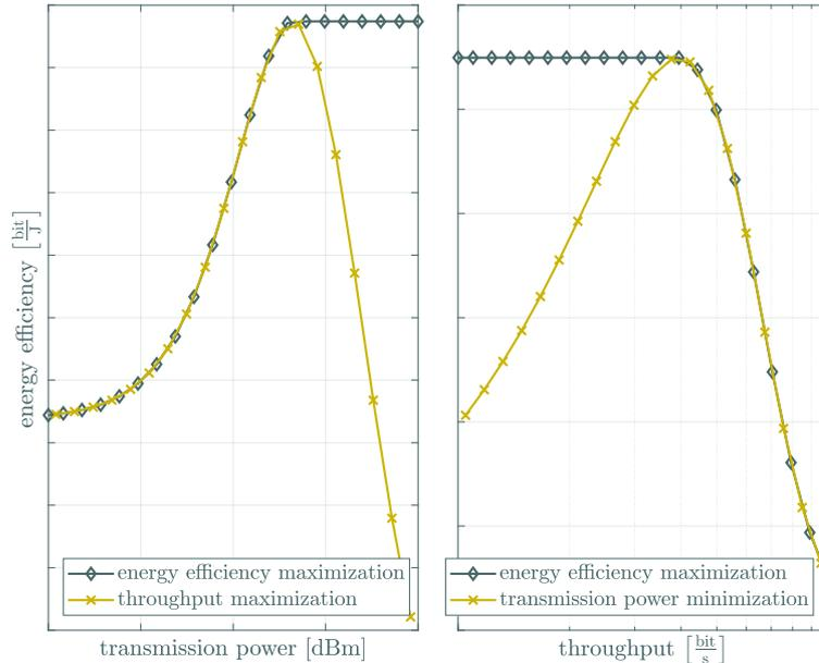
Figure 2.3: The energy efficiency as a function of available transmission power for the EE and throughput maximization (left subfigure), or as a function of the minimal throughput for the EE maximization and transmission power minimization (right subfigure).
