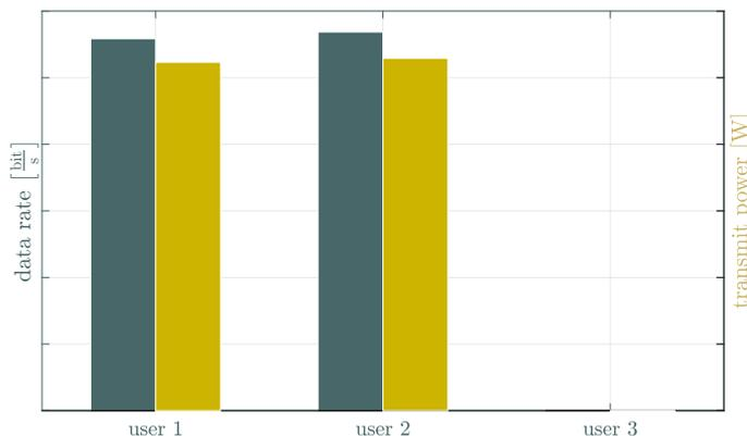
Figure 3.3: The data rates and transmit powers of three users in the network where two of the users are located close to the base station while the third is located at the edge of the cell. The case of EE maximization without additional constraints.
