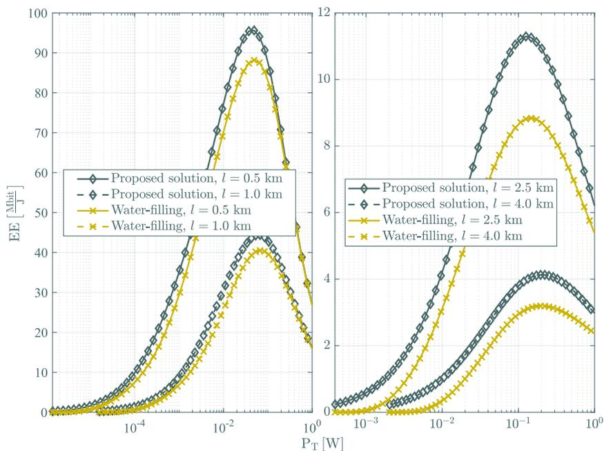
Figure 2.8: Energy efficiency versus the total transmit power.
