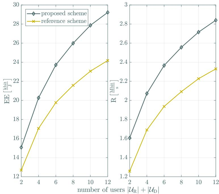
Figure 4.15: The energy efficiency and throughput versus the number of users.
