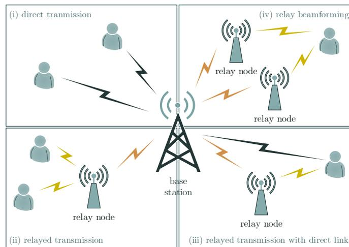
Figure 4.1: The transmission modes in the multiuser OFDMA relay network.
