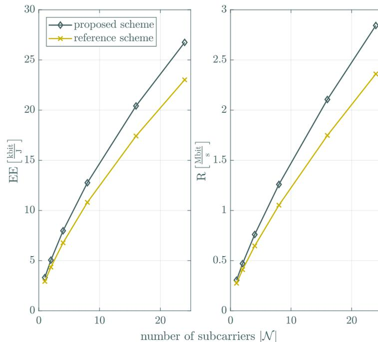
Figure 4.13: The energy efficiency and sum-throughput versus the number of subcarriers.
