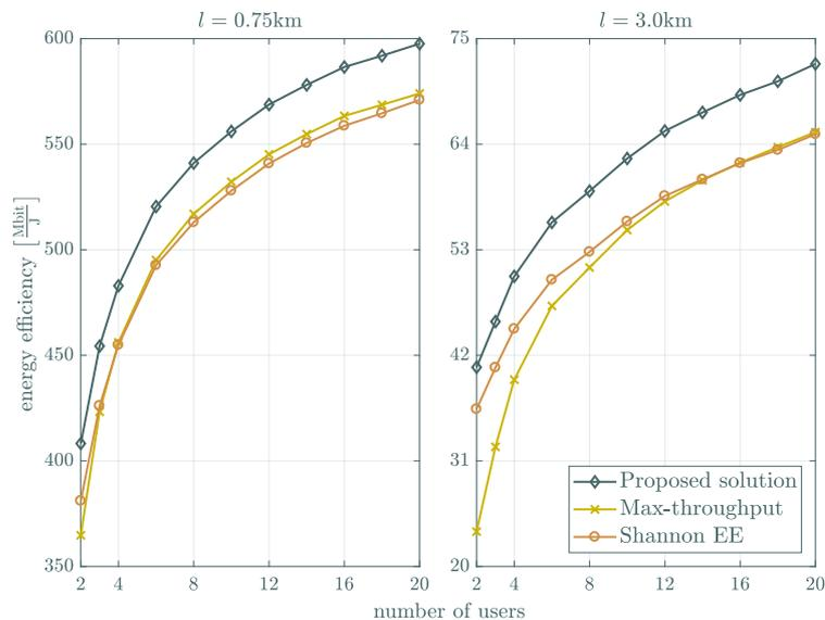
Figure 3.8: energy efficiency versus the number of users for  $l = 0.75\text{km}$  (left) and  $l = 3.0\text{km}$  (right).
