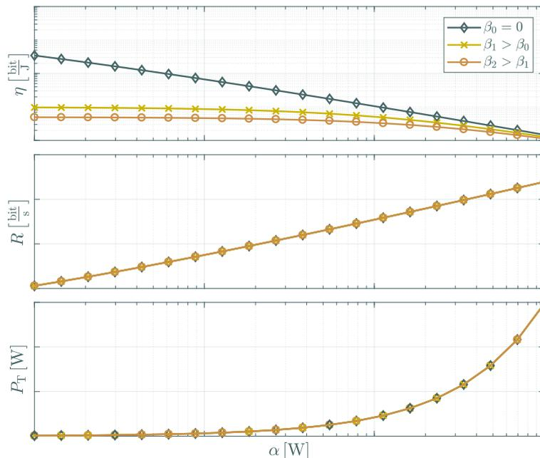
Figure 2.2: The energy efficiency, the data rate and the transmit power as a function of the static part of the circuit power  $\alpha$  for different values of parameter  $\beta$  related to the dynamic part of the circuit power consumption.
