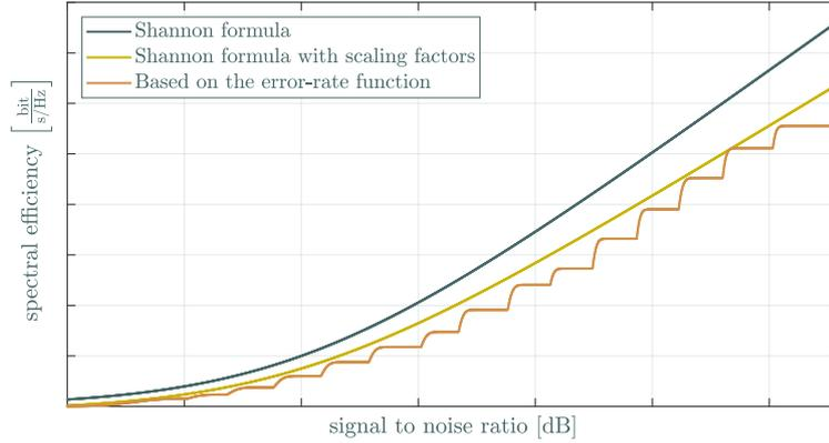
Figure 1.3: The spectral efficiency as a function of SNR for three approaches of the data rate estimation.
