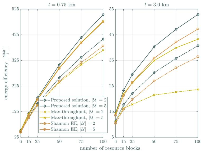
Figure 3.6: Energy efficiency versus the number of available RBs for  $l = 0.75\text{km}$  (left) and  $l = 3.0\text{km}$  (right).
