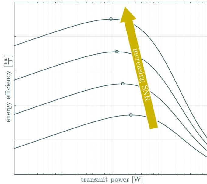
Figure 1.1: Relation between the EE and transmit power for different values of the SNR.
