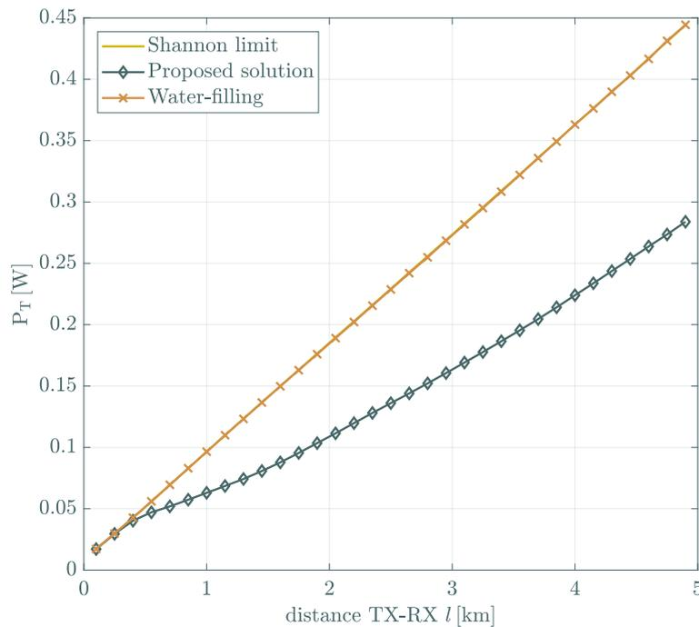
Figure 2.6: Total transmit power versus the link distance.
