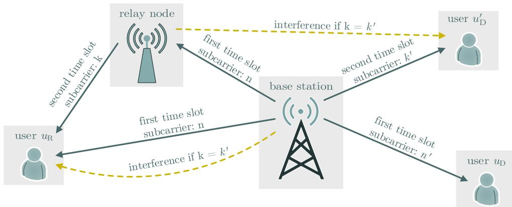
Figure 4.8: Exemplification of the relayed and direct transmission modes using two time slots and subcarriers:  $n$ ,  $k$ ,  $n'$  and  $k'$ .
