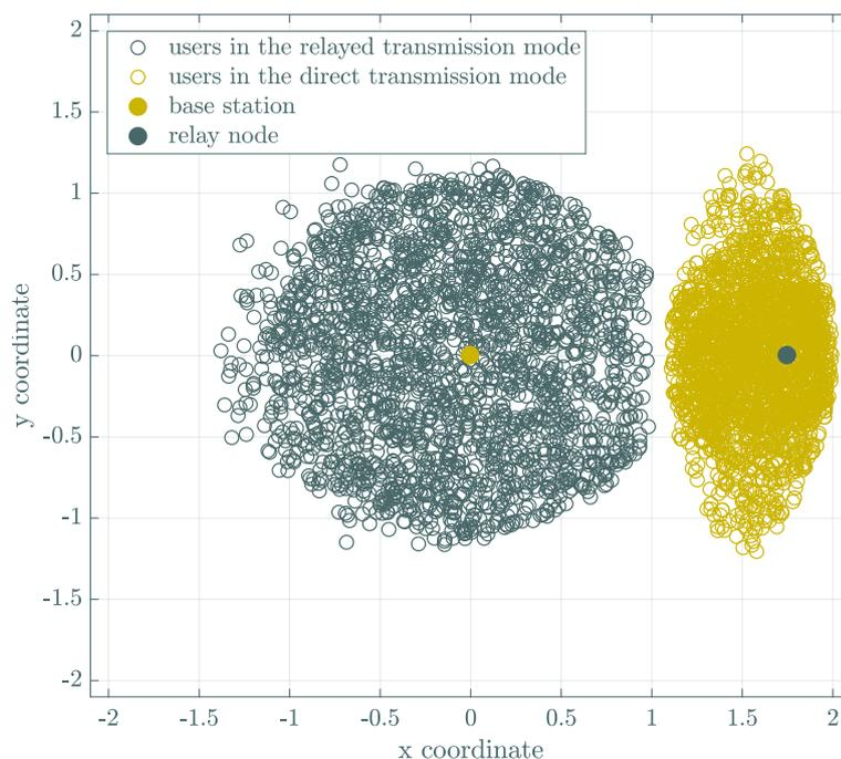
Figure 4.11: The cases when the same subcarriers are obtained for the direct and the relayed transmission in the second time slot.
