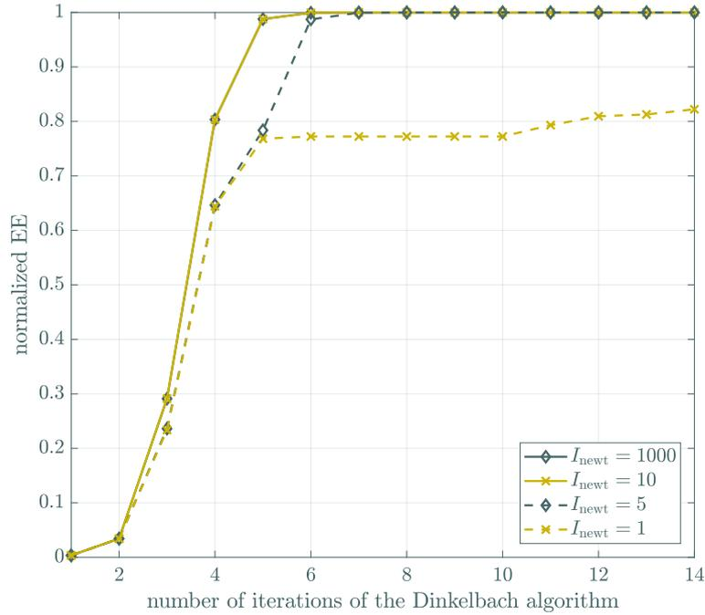
Figure 4.10: The normalized energy efficiency metric as a function of number of iterations of the Dinkelbach method.
