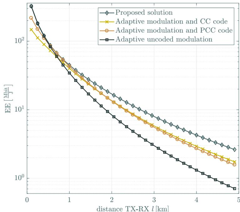
Figure 2.7: Energy efficiency versus the link distance.
