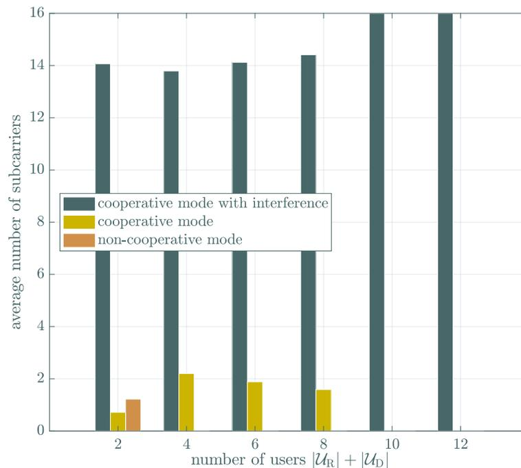
Figure 4.16: The mean of subcarriers used in a given transmission mode versus the number of users.
