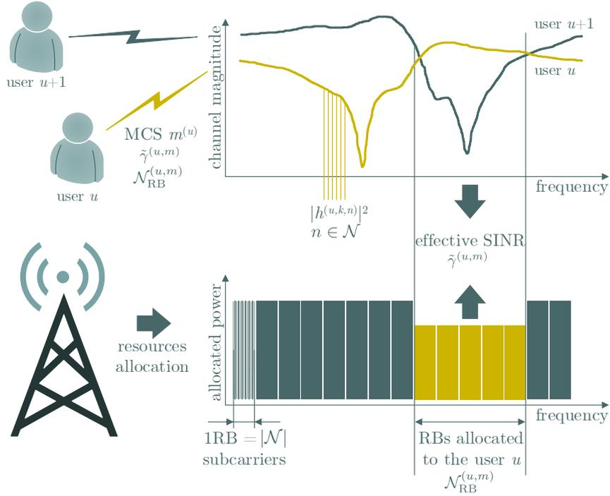
Figure 3.4: System model with MCS and power allocation for RBs of distinct users in the downlink.
