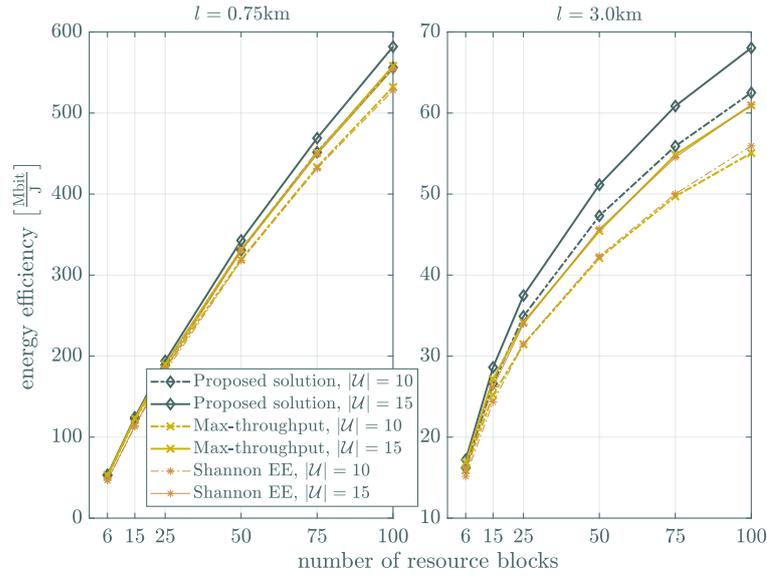
Figure 3.7: energy efficiency versus the number of available RBs for  $l = 0.75\text{km}$  (left) and  $l = 3.0\text{km}$  (right).
