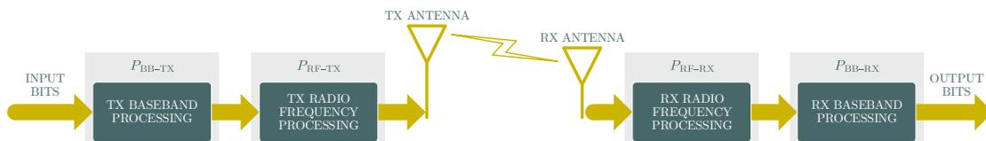
Figure 1.5: The general block diagram of the transmitter and receiver with the power consumption description related to each element.
