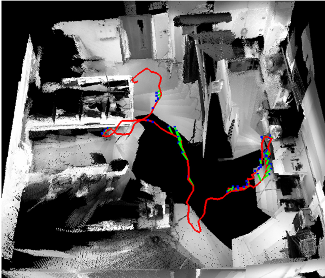
Fig. 10. Global localization results for the PUT RGB-D/Workshop data set seq2 for \tau_{\text{prob}} = 1.0 , \tau_{\text{res}} = 0.07 , and \tau_{\text{div}} = 6 . Test trajectories are marked with red lines, recognized places with blue dots, while green lines connect the recognized locations to their respective ground truth poses (for interpretation of the references to color in this figure legend, the reader is referred to the web version of this article).
