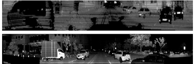
Fig. 4. Visual comparison of intensity images quality from Velodyne HDL-64E (top) and Ouster OS1-64 (bottom) showing that using intensity data from the KITTI dataset might not bring significant benefits.
