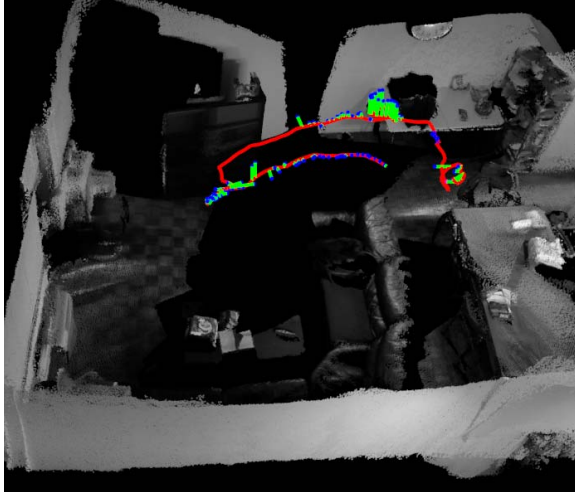
Fig. 6. Global localization results for the NYUv2 dataset for \tau_p = 1.2 , \tau_{pd} = 0.2 , and \tau_s = 0.03 . Test trajectories are marked with red lines, recognized places with blue dots, whereas green lines connect recognized locations to their respective ground truth poses
