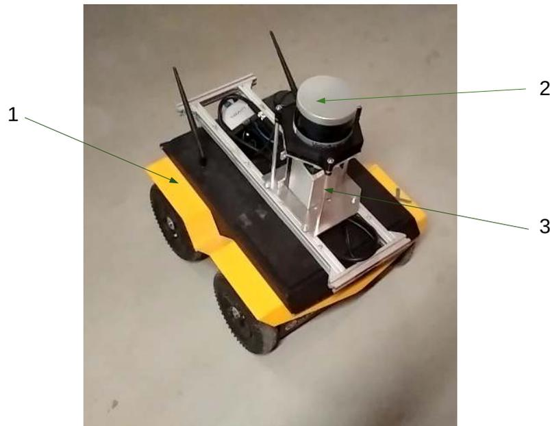
FIGURE 5.12: A robotic platform used. 1- Clearpath Jackal mobile robot, 2- Velodyne VLP-16, 3- Livox Lidar with planar reflectors.
