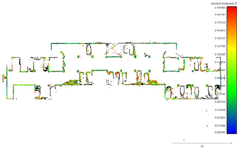
(A) Comparison between investigated LiDAR and ground truth.
