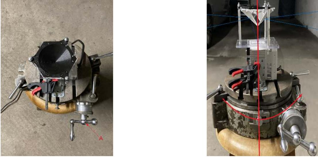
FIGURE 4.13: The experimental prototype mounted onto a precise rotating table during the data acquisition procedure. 'A' marks the axis for changing the rotation angle.
