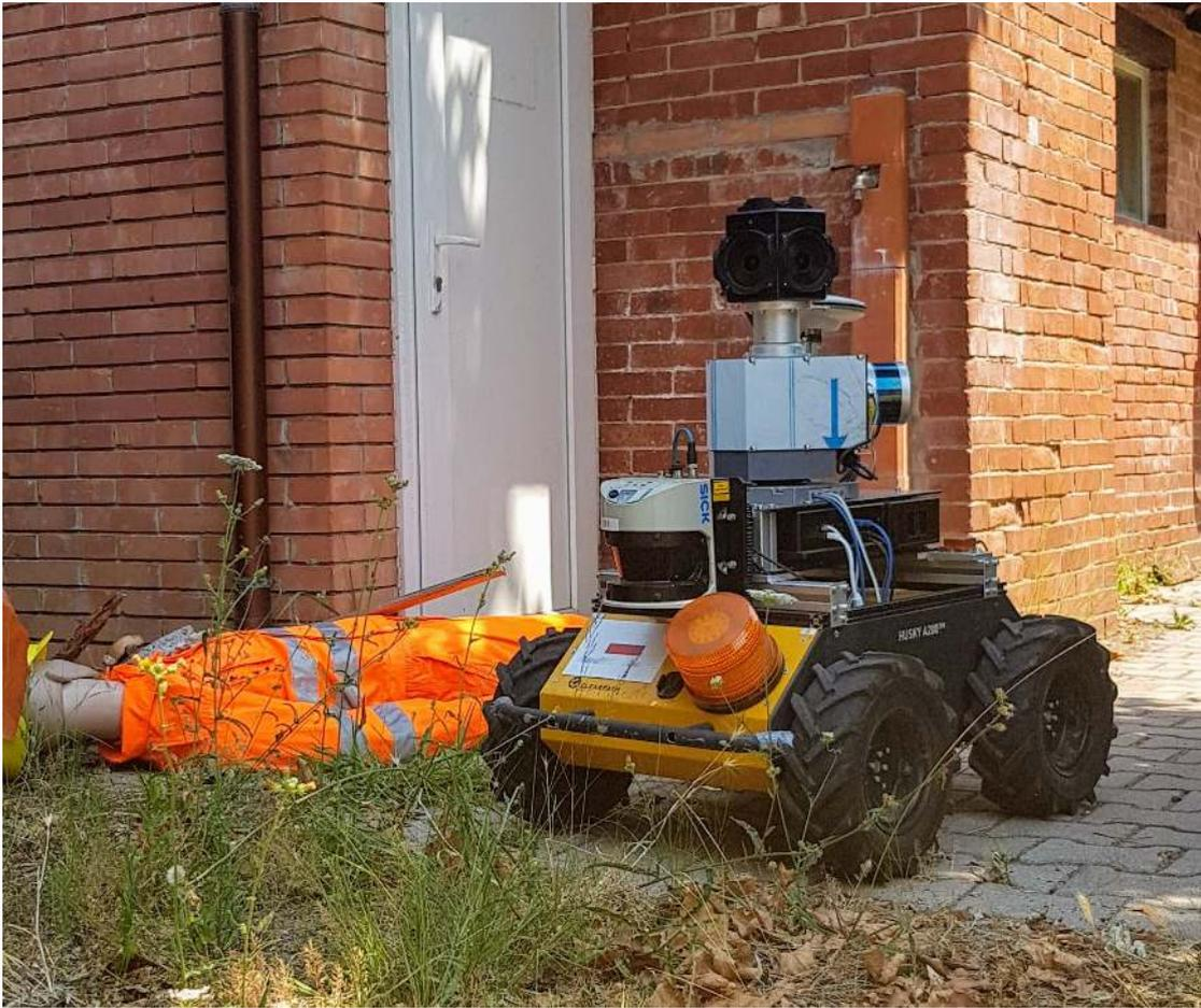
(A) 3D unit mounted on top of mobile robot during simulated search and rescue scenario.
