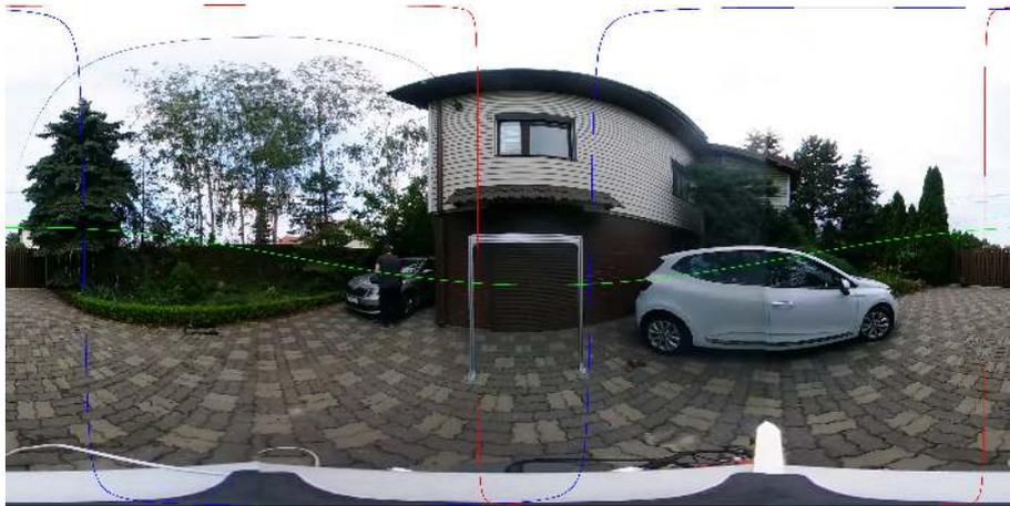
FIGURE 4.33: Pre-calibrated image with projected lines feature which were detected in the point-cloud.
