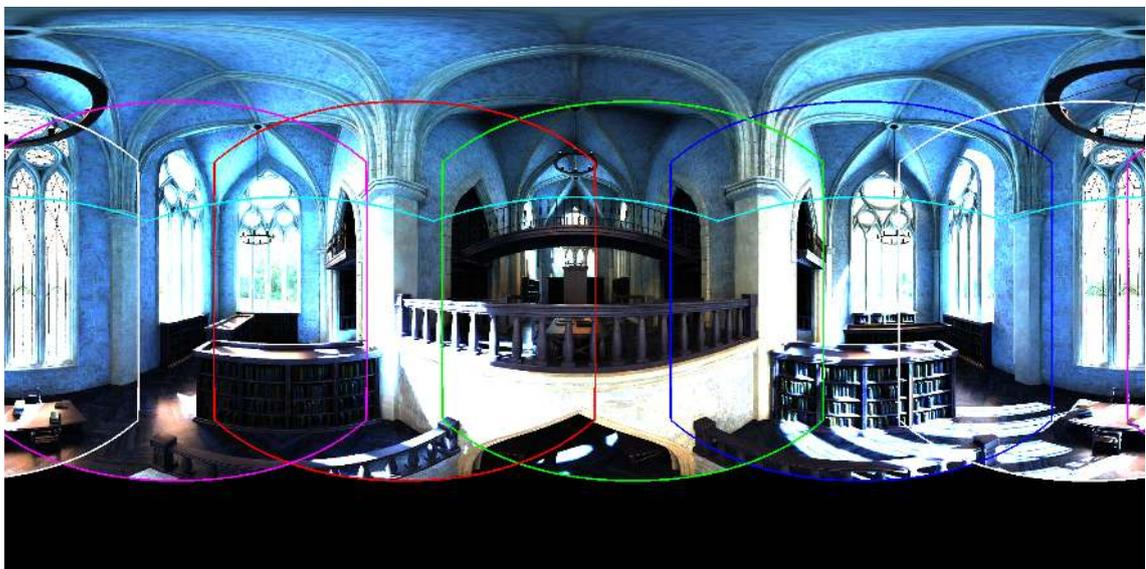
FIGURE 1.5: Panorama rendered with six camera rig from figure 1.2, projected on sphere with radius 10 meters. Projected field of view boundaries are marked in color.
