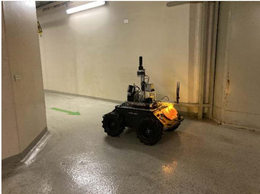
FIGURE 5.6: Robotic mapping system used for the scenario.
