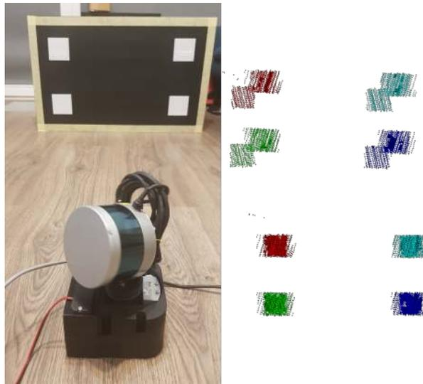
FIGURE 4.25: Left - photo of the calibration pattern, right top - projection of detected patterns using initial (CAD) calibration, right bottom - projection of detected patterns using optimized calibration.
