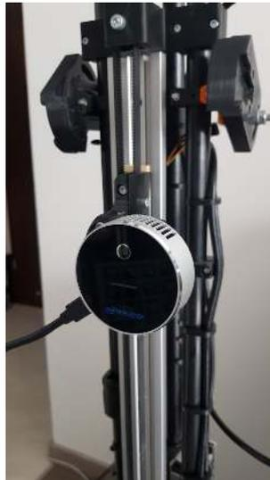
FIGURE 4.5: One of the two scanning heads. There is a visible guiding system with a timing belt in the back. In the front, there is an RGBD sensor with an RGB camera and LiDAR lens.
