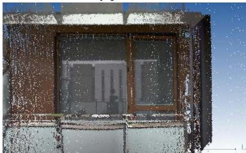
(C) Image point-cloud, sphere stitched for sphere 2m.
