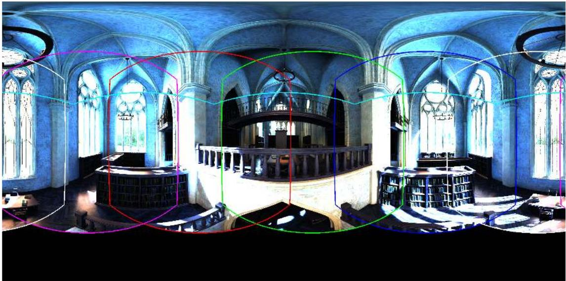
FIGURE 1.4: Panorama rendered with six camera rig from figure 1.2, projected on sphere with radius 2 meters. Projected field of view boundaries are marked in color.
