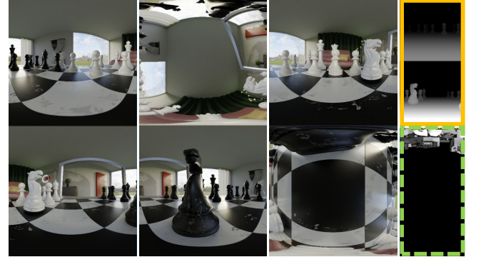
Fig. 5: Example of four atlases produced by MIV encoder in the proposed methods: three texture atlases and one depth atlas: IDMA – only the yellow part, eIDMA – entire depth atlas (yellow and green parts).
