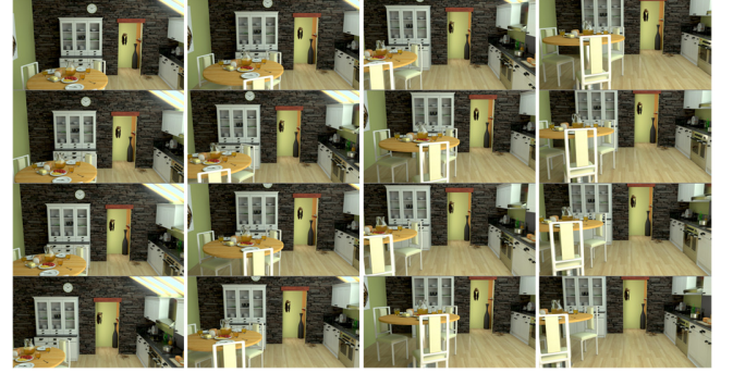
Fig. 3. Example of four atlases produced by MIV encoder running in MIV Geometry Absent profile: all four atlases contain full views.
