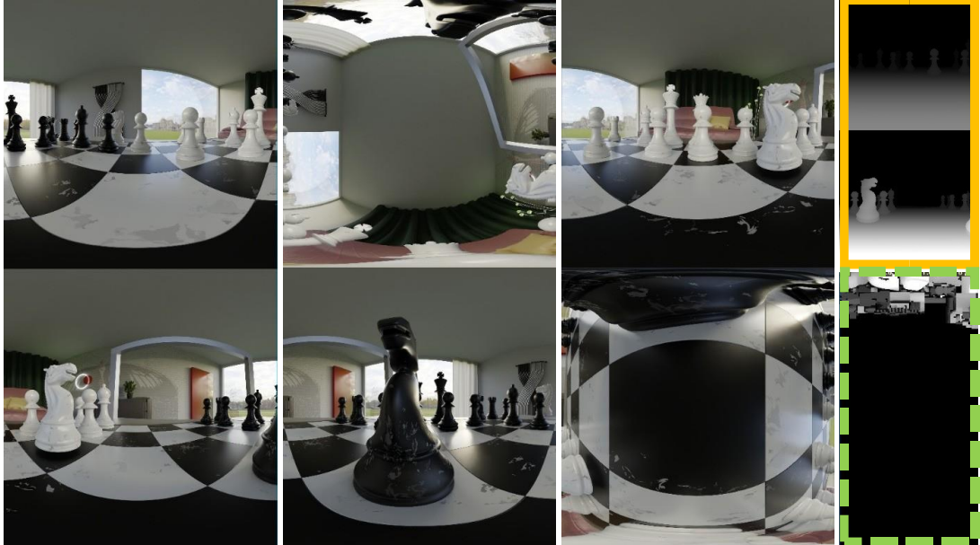
Figure 4.1.2. Example of four atlases produced by MIV encoder in the proposed methods; IDMA – three texture atlases and only the yellow framed part of the depth atlas, eIDMA – three texture atlases and both yellow and green bordered parts of the depth atlas.
