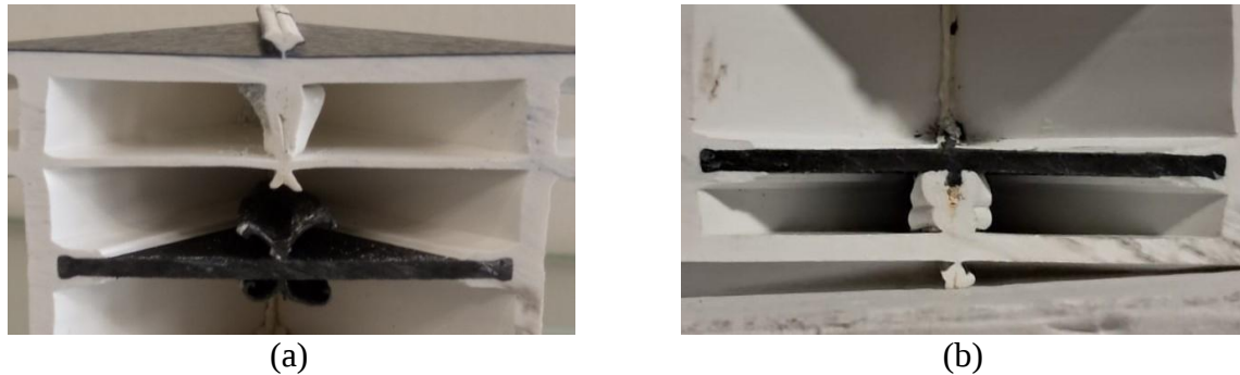
Fig. 4.105. Cross-section of the welded profile showing the composite insert arrangement: (a) variant without composite milling, (b) milling of the composite insert to a depth of 1 mm. Source: Author's own work
