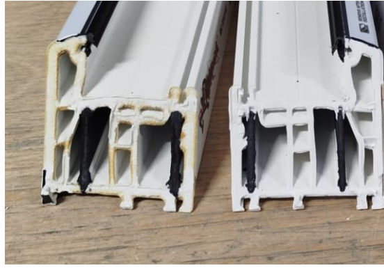
Fig. 4.106. Cross-sections of welds produced at 270 °C (left profile) and 264 °C (right profile). Source: Author's own work
