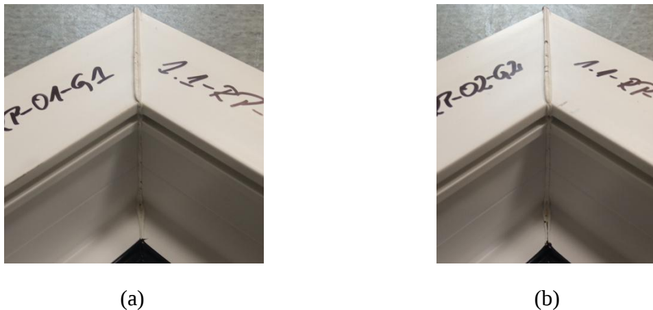
Fig. 4.44. Representative welds from the reconnaissance tests: (a) specimen welded using the first head, (b) specimen welded using the second head [13]
