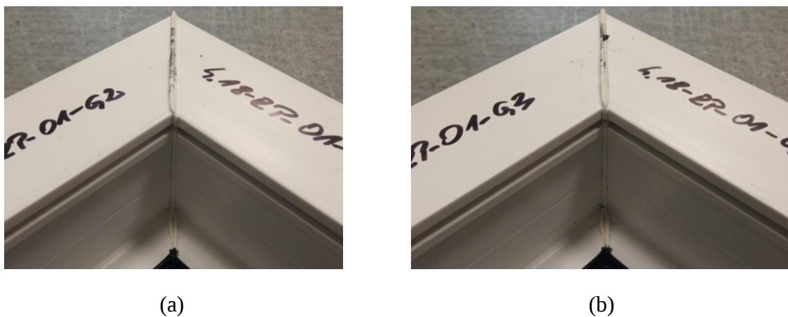
Fig. 4.102. Representative welds from the preliminary trials: (a) second head, (b) third head. Source: Author's own work
