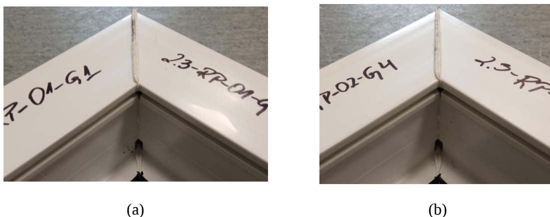
Fig. 4.46. Selected welds from test specimens produced with composite milling to a depth of 6 mm: (a) welded using head 1, (b) welded using head 4 [13]
