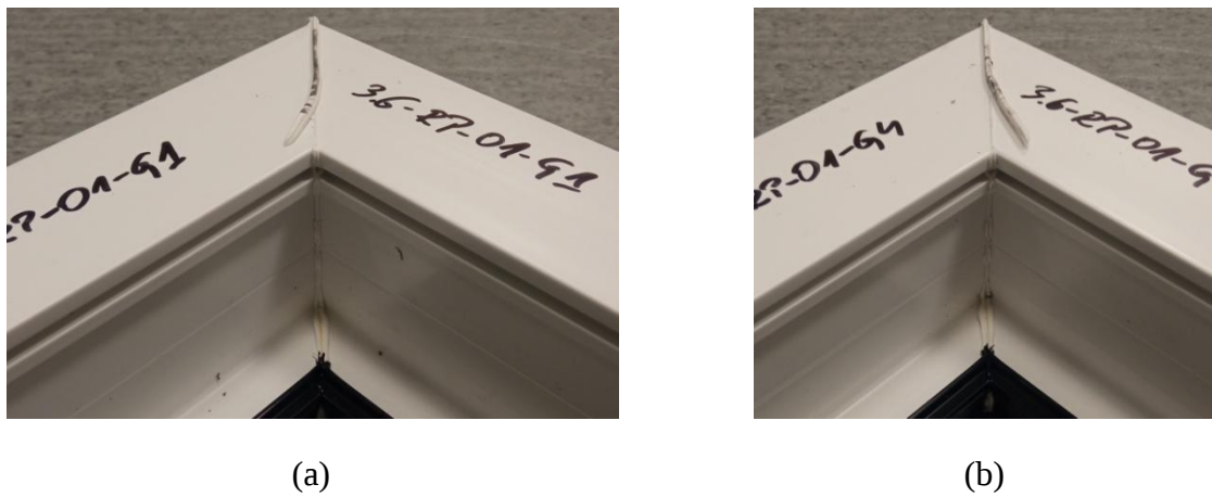
Fig. 4.69. Representative welds from the reconnaissance tests: (a) welded using head 1, (b) welded using head 4 [12]
