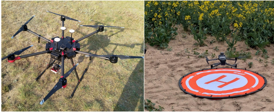
Figure 2.5: Examples of UAV platforms used for multispectral data acquisition: a DJI Matrice 600 Pro equipped with an external MicaSense multispectral camera (left), and a DJI Mavic 3 Multispectral with an integrated multispectral sensor (right).
