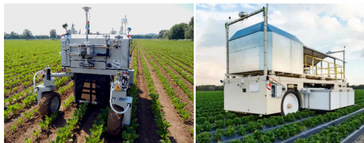
Figure 2.7: Examples of ground-based robotic platforms for agricultural applications. Left: BoniRob used for weed control (image from [38]); right: Harvest CROO robot with manipulators to pick strawberries (image from harvestcroorobotics.com website).
