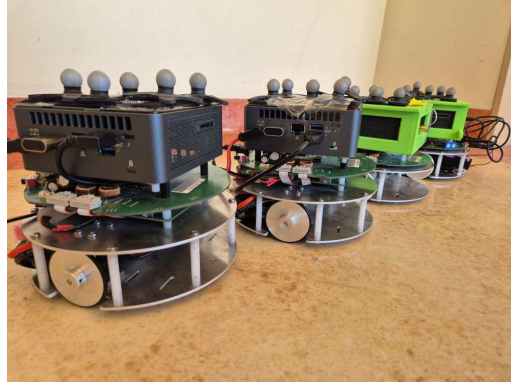
Figure 3.13 – The mTracker mobile robots, equipped with the Intel NUC computers, which were used to create a multi-vehicle system for the purpose of experimental tests.
